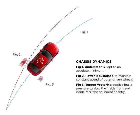
Also, to help XE tackle winding roads, there's intelligent Torque Vectoring by Braking technology. On tight turns, it applies the brake to the inside wheel and directs more rotating force from the engine to the wheel with the most grip. The result is an exceptional combination of sports car-like agility, more consistent road holding and a feeling of added confidence when you're driving.
